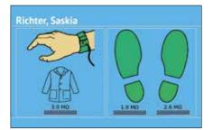
Shoes and wriststraps can be tested simultaneously. Configurable measuring voltage and thresholds enable optimal adaptation to your requirements.
